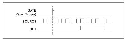
Figure 7-23. Single Pulse Generation with Start Trigger
